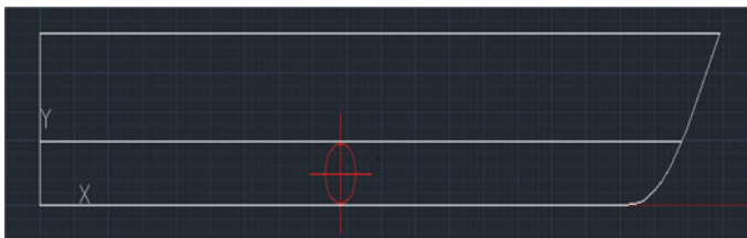
Fig. 12 Position of the anode on the hull
