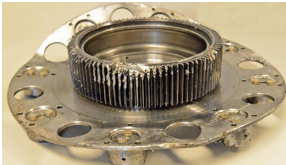
Fig. 1 Recovered epicyclic planetary module from a crash (AIBN 2016)
